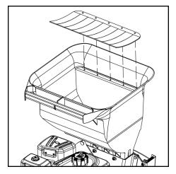
31. The black side of the hopper-guard is considered the top. Insert one (1) #14 x 3/4" Phillips-head, self-tapping screw into each of the five (5) holes located along the top edge of the hopper-guard. This will make it easier to install the hopper-guard and help reduce the chances of dropping a screw into the lower-unit assembly.
