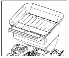
32. Hold the hopper-guard inside the hopper, while keeping the guard's free-end raised slightly, as shown; This will also help reduce the chances of dropping a screw into the lower-unit assembly. Use a Phillips-head screw driver to securely tighten the five (5) screws.
